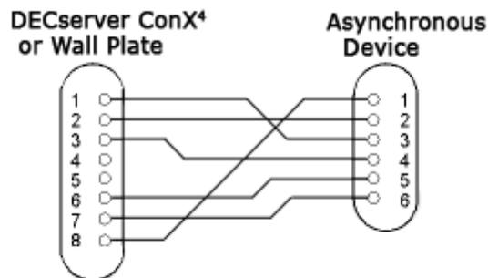
Table A-8 defines the wiring configuration for the BN24H cable.
